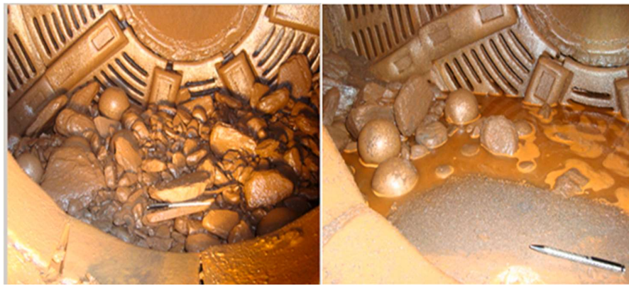
Fig. 7. Typical mill loads as observed in pilot scale tests: open circuit (left) and closed-circuit (right) SAG operation (modified from Rodrigues, 2014).
