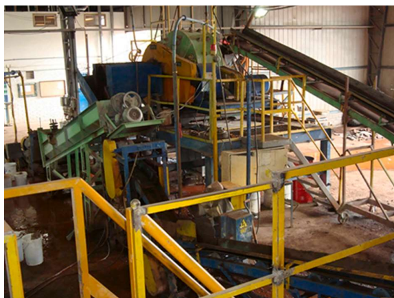
Fig. 3. Overview of the pilot SAG mill, with the spiral classifier on the left (Rodrigues, 2014).
